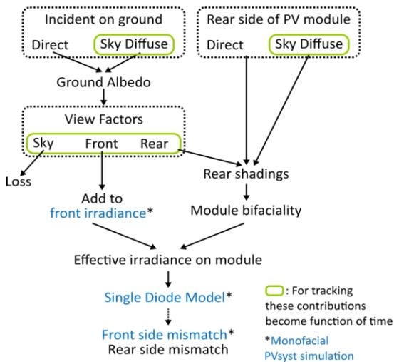
**Figure 2:** Simulation steps for the bifacial model. The blue steps are the interface to a normal non-bifacial simulation. The green steps are the contributions that are constant with fixed orientations and become functions of time with tracking installations.
