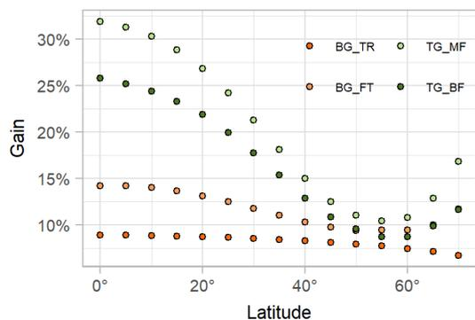
**Figure 7:** Bifacial gain as function of latitude, for clear sky conditions. For each latitude, the orientation of the fixed tilt scenarios was optimized.
