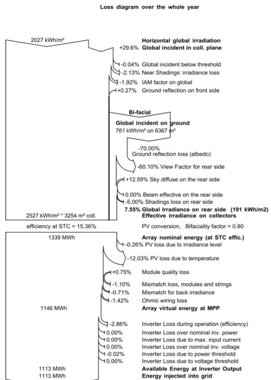
**Figure 3:** Loss diagram for a simulation with bifacial single axis trackers.
