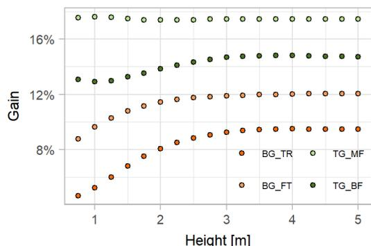
**Figure 6:** Bifacial gain as function of mounting height for the different gain factors.
