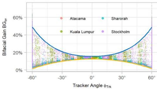
**Figure 9:** Distribution of bifacial gain factor for tracking systems. The blue and yellow curves are approximate, and represent the bifacial gain factor for the diffuse and direct component only.
