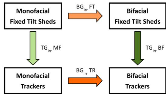
**Figure 4:** Gain factors for irradiance. Green arrows denote transitions from fixed orientation to tracking. Orange arrows denote transitions from monofacial to bifacial PV modules.
