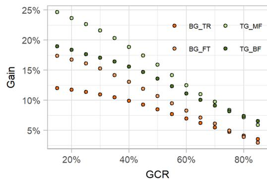
**Figure 5:** bifacial gain as function of ground covering ratio GCR for the different gain factors.
