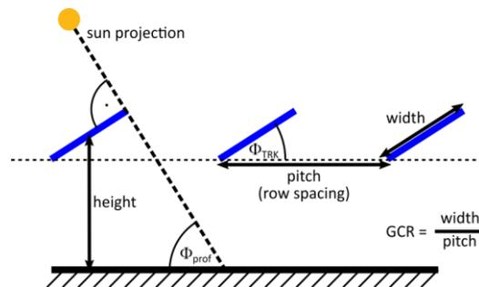
**Figure 1:** Two-dimensional model used for calculating the irradiance that is scattered back from the ground.
